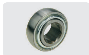
G22097 OEM No.:AA22097 205KRRB2 Weight:0.40 lbs Bearing with 7/8" hex bore. Has curved O.D., used on seed and fertilizer drives. Replaces JD No. AA22097.
