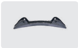
G261140 OEM No.:N261140 Weight:9.7 lbs Shank protector for curved shank with shear bolt or standard spring reset. Fits John Deere rippers 512, 913, 915, 955, 2700. Requires 2 mounting holes on 11-1/4" centers. Chrome-Nickel construction for longer wear.
