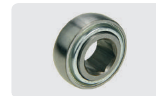
G22097 OEM No.: G2100-03 Weight: 0.4 lbs Bearing, 7/8" hex bore, curved outer race, 7/8" inner race width. Used on Kinze planter seed and fertilizer transmission, hex drive lines, contact drive wheel.
