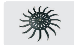
G142664 OEM No.: AN142664, 3400-111 Weight:16.70 lbs John Deere Rotary Hoe Wheel, 21" Diameter.16 curved tines with heat treatment , fits for John Deere Tillage(s) 75, 415, 420, 428, 430.
