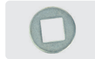
G16690 OEM No.:A16690 Weight:0.15 lbs John Deere washer for cast iron bumper. Axle washer, 3/16" thick, 1-1/8" square hole. 2-1/2" O.D.
