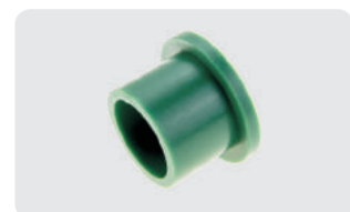
G817-084C OEM No.:817-084C Weight:0.01 lbs Green nylon pivot bushing. Fits late model drills with single opener arm, 2 used per row; 8 used per row on models with parallel arms; also used on press wheel arm on late models. Fits Yield Pro planter row unit. 3/4" I.D., 61/64" O.D., 1-1/4" flange O.D., 13/16" long. Replaces Great Plains No 817-084C.
