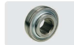
W210PP4 OEM No.: W210PP4, DC210TT4, 7AS10-1-1/8, 10446, 10778, NH86548582 Weight: 2.05 lbs Disc Harrow Bearing - 1-1/8" Square Bore - Replace: BCA/FEDERAL MOGUL: DC210TT4 FAFNIR/TORRINGTON: W210PP4 NDH: AS4510B NTN: 7AS10-1-1/8 DIMENSIONS: BORE: 1-1/8" SQUARE O.D. 90MM FLAT
