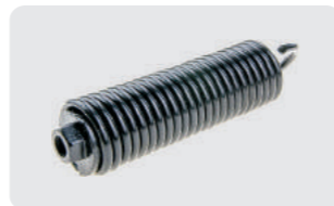
G10071 OEM No.: AB10071 GA2052 FC6108 Weight: 1.05 lbs Down pressure spring with plug for John Deere 7000, 7100, and Kinze Row Unit. Will replace JD AB10071, Kinze GA2052. coil length is 4 3/4" oal lth is 6 1/4". 3/8" bolt thread, Fits Maxemerge®, Kinze prior to 1989 and White early 6000 series.
