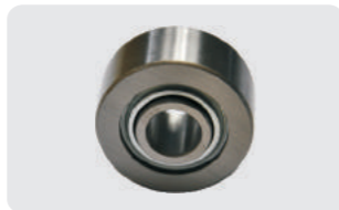
G35638 OEM No.:203KYP2 AA34132 AA35638 Weight:0.61 lbs John Deere Closing wheel bearing for John Deere planter 7200,7300 and IHC model 296 & 386 planter, Bore Size:0.669" Round, O.D.:1.574" flat, IR width:0.55", OR width:0.472".
