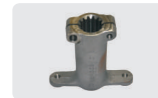
G34359 OEM No.:R34359 Weight:1.36 lbs John Deere Hydraulic Pump Drive Shaft bHydraulic Pump Drive Coupler, 14 Spline, Length - 4.37". Fits John Deere Tractors - 3020, 4000, 4020, 5010, 5020 Industrial/ Construction - JD440, JD500, JD500A, JD600, JD760
