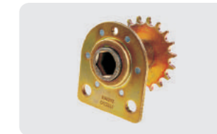
G36212 OEM No.: AA36212 Weight: 1.3 lbs Bearing with 19 tooth sprocket, 7/8" hex bore, 2-1/8" width. Used on 7200-7300 and 1700 series planters row unit and planter drive line. Replaces JD No. AA36212.
