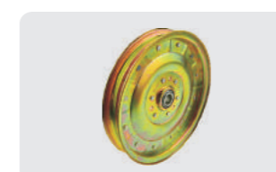
G97031 OEM No.: AH97031, 71135623,674966R91, 1033064M1,76288, 7530070,31-1588690 Weight: 3.28 lbs John Deere flat flanged idler, replaces John Deere AH97031, AGCO No. 71135623,CASE-IH No. 674966R91, MASSEY No. 1033064M1, New Holland No. 76288 and White-Oliver No. 7530070,31-1588690 O.D.:8-3/4" I.D.:5/8" WIDTH:1-7/16"
