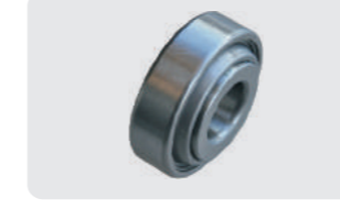
G10448 OEM No.:205KP8 ,JD10448, JD9331,205KR3, 669807C91 Weight:0.30 lbs the ball bearing fits on John Deere and IH coulter wheels, IHC cotton picker & Lilliston carry wheels. Bore size: 0.751", O.D.size:2.047 " flat, IR width: 0.64" and OR width: 0.70".
