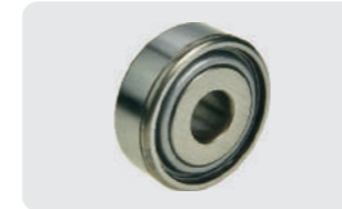
205DDS-3/4 OEM No.:205DDS-3/4 188-007V Weight:0.49 lbs Great Plains Grain Drill Disc Bearing,205 Series Row Unit Disc Bearing for Great Plains. Replaces Great Plains 188-007V. Has gothic arch and triple lip seal. Replacement bearing only for seed opener assembly. Has 3/4" round hole in center.
