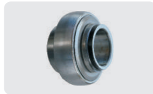
G214862 OEM No.:AH214862, 205-100-2RFW,JD9273, AH169077 Weight:0.55 lbs John Deere Ball Bearing, Shoe Grain Supply Auger AH214862. Double extended inner, Spherical outer. I.D. 1.00" (25.40mm), O.D. 2.047" (52mm), Width 1.750" (44.45mm). For various combines.
