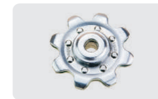
G102448 OEM No.: AN102448 Weight: 1.47 lbs Lower Idler sprocket, non-greasable 8 tooth, 5/8" bore, sealed bearing. John Deere, fits all 40 series to s/n 466450, also fits 235, 335, 435, and 635. Replaces JD No. AN102448. Case-IH, fits 900-1000 Series. New Holland, fits all 974 series. Replaces NH No. 573399.
