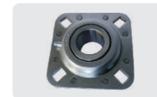
FD209RB OEM No.:FD209RB Weight:3.31 lbs 1.5" Riveted Flange Disc Harrow Bearing-Replaces 1934-12-0, FD209RB. Krause Disc Harrow BCA/FEDERAL MOGUL: FD209RB FAFNIR/TORRINGTON: DHU1-1/2R-209 FAFNIR: DHU112R209 KRAUSE: 1934-12-0 KRAUSE: 40-109 WHITE: 238813B DIMENSIONS: BORE: 1-1/2" ROUND BOLT TO BOLT: 5" (BOTTOM LEFT TO TOP RIGHT)
