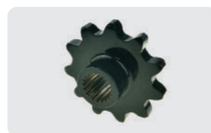
G101339 OEM No.:AH101339 Weight:1.74lbs Drive Sprocket.11-tooth, spline bore. 1 per row on right gathering chain drive. For John Deere 50A series row crop heads.
