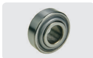
G13975 OEM No.:CJ13975 Weight:0.29 lbs Ball bearing, ID:15mm OD:42mm Width:22mm
