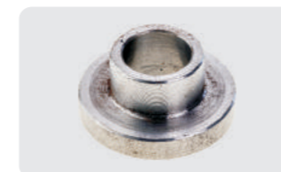
G145044C1 OEM No.: 145044C1 Weight: 0.14 lbs "CIH bushing. 16.5mm IDx38mm OD x 17.5mm L. Fits CASE IH CULTIVATOR 183.
