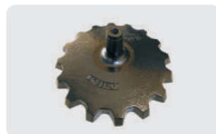
G105392 OEM No.:A105392 Weight:15.97lbs Drill Cruiser Wheel.Angular tooth design helps prevent clogging and provides both sidewall crumbling and soil firming action. For John Deere 1560, 1590, 1690,1860, 1890, 1895, 1990 drills, air seeders.
