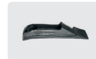
G801400 OEM No.:TF801400 Weight:15.98 lbs Blue Jet replacement fall point. This point is made of a chrome cast material reinforced with Nickel for longer wear. 2-7/8"X15-1/2"
