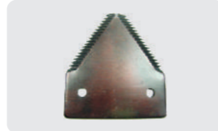
G158516 OEM No.:158516,102053 Weight:0.15 lbs Sickle section, black, 7 teeth per inch. Fits MacDon platforms 960, 962, 963, 972, 973, 974, D50, D60, FD70, FD75. Case-IH platforms 1042, 1052, 2042, 2052, 2062. 2142, 2152, 2162. New Holland platforms 84C, 86C.Width 3", Hole Spacing 2-1/8",Length 3-1/4" Replaces MacDon No 102053, 158516.
