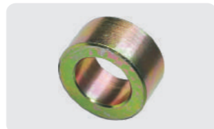
G48515 OEM No.: A48515 Weight: 0.1 lbs Pivot bushing for parallel arms. Replaces JD A48515 Applications: For Front and Rear upper parallel arms and front lower parallel arms on MaxEmerge® 2 size:0.658"x 1.084"x0.568".
