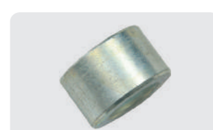
G137512 OEM No.: 137512C3 Weight: 0.075 lbs Bushing for for 3/8" thick parallel arms. 13.5mm ID x 22.23mm OD x 13.5mm L.For Case-IH 800, 900, 950, 955, 1200 series planters; 5400, 5500 Soybean Special. Replaces Case-IH No 137512C3.
