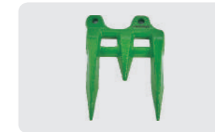
G213405 OEM No.: H213405 Weight:2.05 lbs Long-short-long standard guard. Fits John Deere 600D, 600R, 925D, 930D, 936D rigid grain platforms. Long point guards comb and lift the crop for even cutting, improving platform productivity. Since this guard has two long points, it is more susceptible to breakage than the H213508 with one long point.
