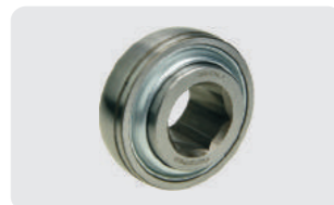
GW211PP27 OEM No.: GW211PP27 DC211TTR27 Weight: 2.71 lbs Disc Harrow Bearings - 1-1/2" Square Bore - Replace : AMCO: G12233 BCA/FEDERAL MOGUL: DC211TTR27 FAFNIR/TORRINGTON: GW211PP27 DIMENSIONS: BORE: 1-1/2" SQUARE O.D. 100MM FLAT, Relube
