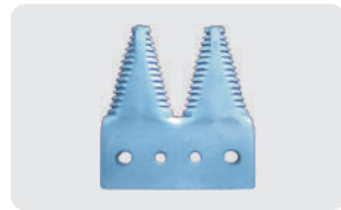
G71353125 OEM No.: 71353125 BDC6700B Weight: Big tooth section to fit 1 1/2", 2 point cutting systems. Section measures 3" wide. The bolt holes are slotted to fit both 2" bolt spacing and 2-1/16" bolt spacing. This section has 7 serrations per inch and is chrome plated. This section will also work on spliced Double Cut 2 sickles because it has the 2 extra holes for the splice area. This section is also commonly used on Agco Clean Cut cutting systems. Replaces Agco number 71353125.
