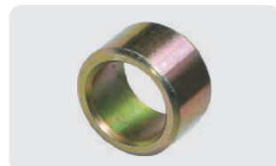
G23789 OEM No.: A23789 GB0218 Weight: 0.04 lbs Bushing for parallel upper and lower arms on JD 7000 and Kinze. Replaces JD No. A23789 & Kinze GB0218. 875" OD, .65" ID, .58" long.
