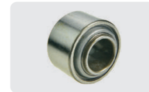
5206KPP3 OEM No.: 5206KPP3 GA8603 Weight: 1.09 lbs Kinze coultter hub bearing for GA5641 hub. All late models. Bore size: 1.187" round, O.D: 2.44" Flat, IR Width: 1.968", OR width: 1.456".
