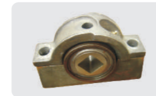
G2951 OEM No.:B2951 Weight:28.65 lbs Bearing with housing,fits 2000 series Pawt 214ra disc. 2-1/4" square axle.replaces Kewanee No. B2951, timken No. Pawt 214ra.
