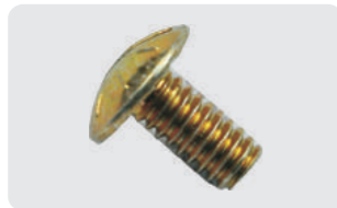
G47782508 OEM No.:477-82508 Weight:0.011 lbs UAR Bolt - serrated slotted truss head, 1/4 NC x 1/2 inch
